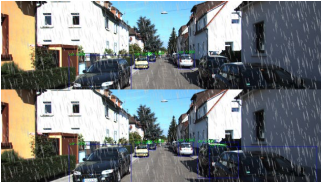
Figure 2. The object detection results of the original FCOS and B-FCOS on rainy days.
