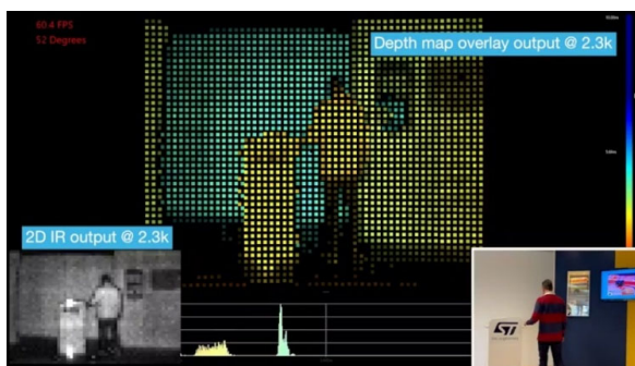
Figure 1. STMicroelectronics VL53L9 direct Time-of-Flight (dToF) 3D LiDAR sensor.
